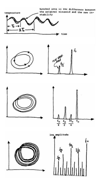
FIG. 2. More figures from reference [8] describe the onset of turbulence through the period doubling cascade. The period of the oscillations doubles with the appearance of an  $f_0/2$ . It doubles again to  $4T_0$  and again to  $8T_0$  as the system becomes increasingly unstable.
