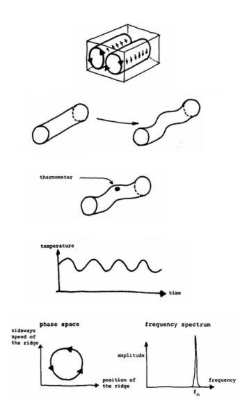
FIG. 1. Two convective rolls form in a finite volume of fluid when it is heated from below. When the heat gradient is very small, the rolling is laminar but when the gradient is increased beyond some critical value the rolls become unstable. When a thermometer is inserted into the cell, it will show that the temperature at the location of the probe oscillates with some frequency  $f_0$ . Figures excerpted from reference [8].
