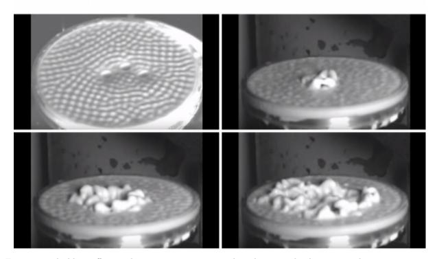
Figure 73: The bloop effect can be seen in experiments such as the one in the this picture where experimenters from the University of Texas at Austin applied extraordinary mechanical accelerations to non-Newtonian fluids. The fluid in this figure is corn starch.
